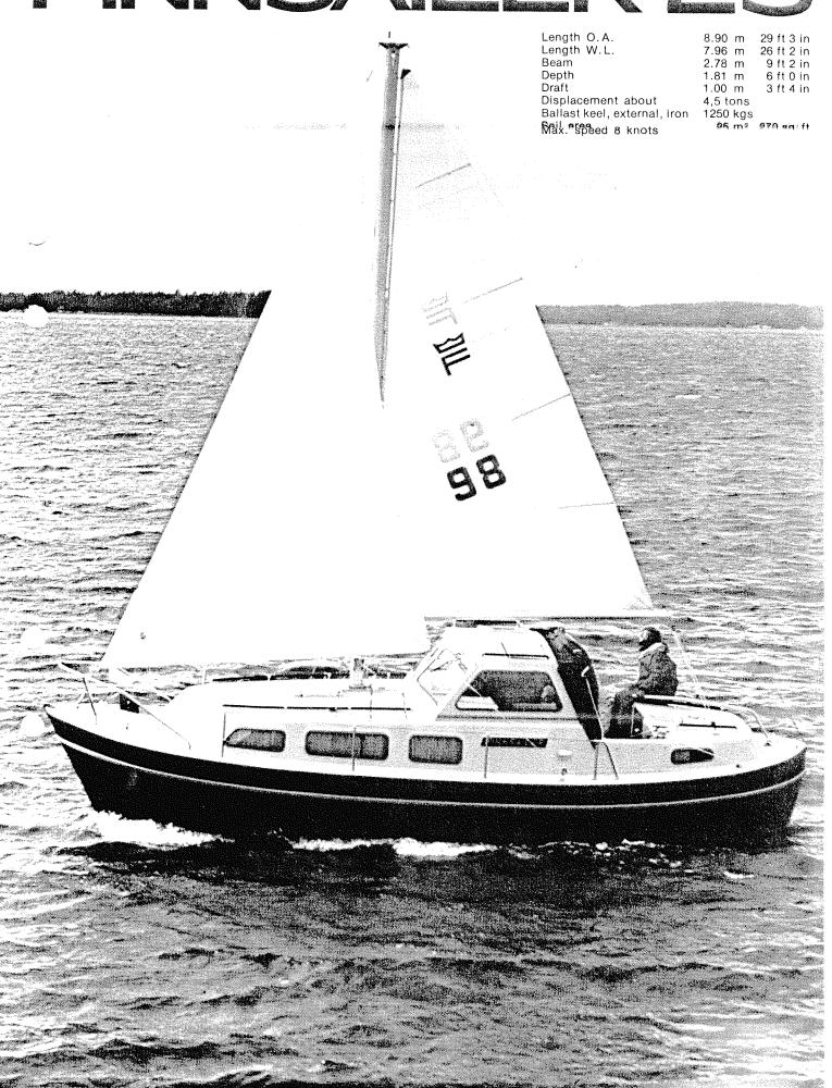
The FINNSAILER 29 motor sailer is a very seaworthy and comfortable boat, built on a traditional fishing-boat hull.
